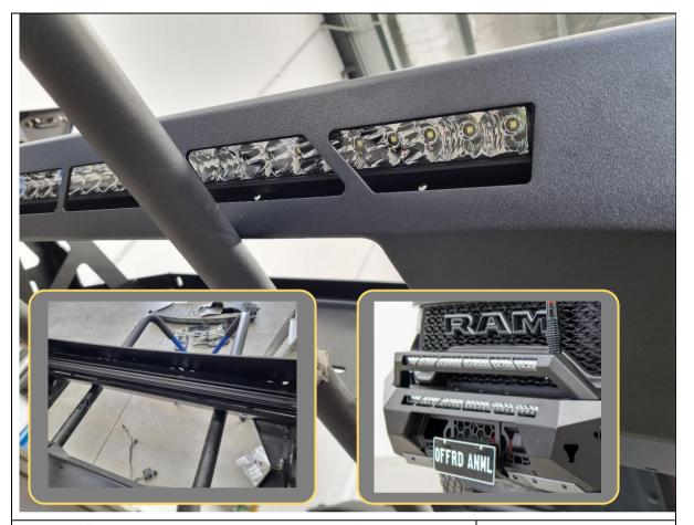
60. If fitting an integrated light bar, do so now from the back.
