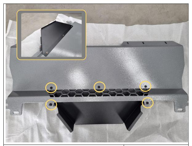
107. Fit the oil cooler air guide to the bash plate as shown, and secure with 5x M6x16 black button head bolts, black washers and flange nuts.
