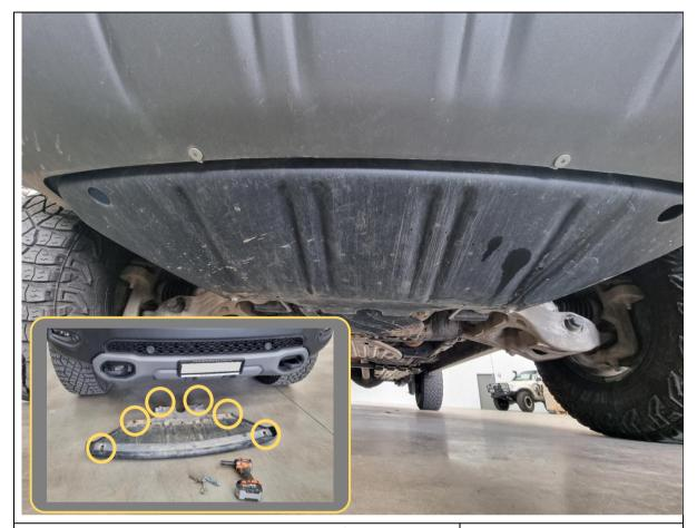
2. Remove 6x 16mm hex bolts holding the factory skid plate.
