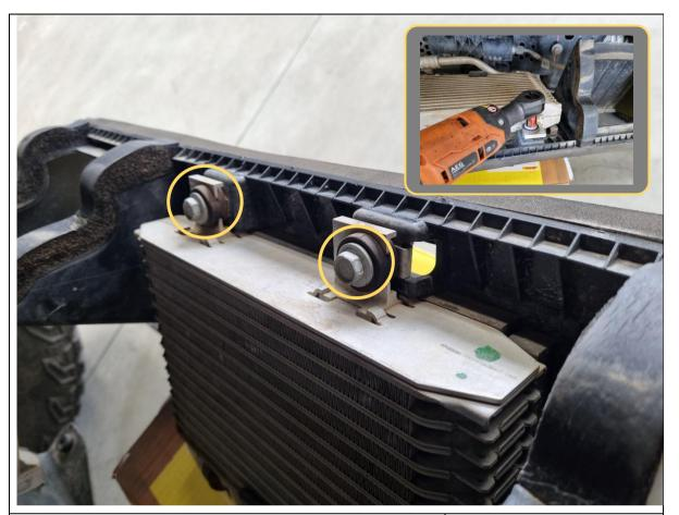
12. Remove 2x 13mm hex bolts holding the top of the oil cooler to its mount. Ensure the rubber parts stay with the oil cooler.
