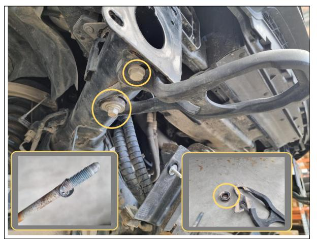
10. Remove 1x 18mm hex bolt (rear) and 1x 21mm hex bolt (front) holding each tow hook to the underside of the chassis. Retain both bolts.
