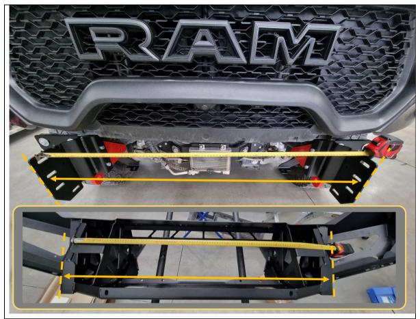
29. Measure the distance between the outside faces of uprights on bar using tape measure. Write distance below for reference if required.
