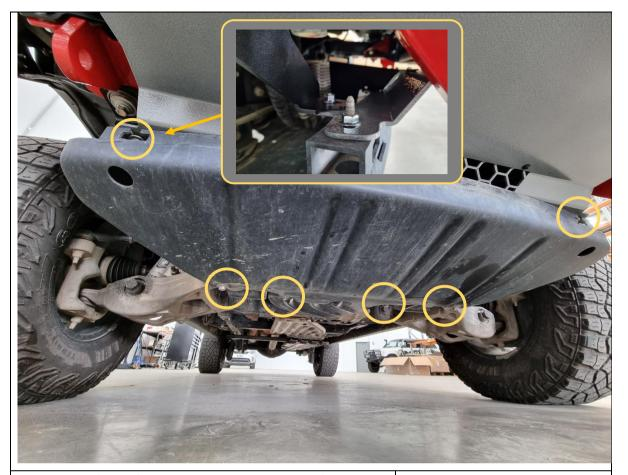
110. Re-fit the factory skid plate, using the 6x factory 16mm hex bolts from Step 2, plus 2x supplied M10 flange nuts for the front 2x bolts into the bash plate.
