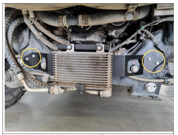
20. Re-use 4x of the 13mm hex bolts from Step 7 and fit the oil cooler and bracket to the embedded nuts in the chassis cross member, as shown.
