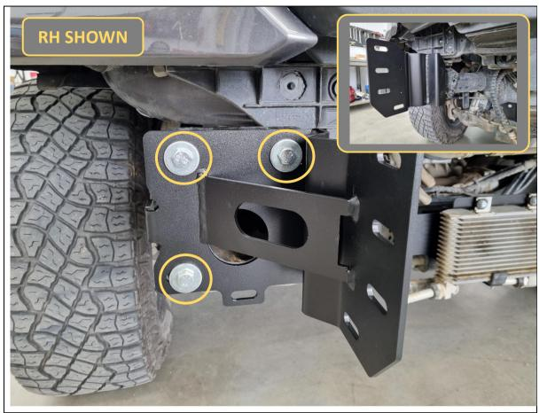
22. Loosely fit each impact assembly to the front face of the chassis horns with 3x M12x30 hex bolts, heavy-duty washers and flange nuts.
