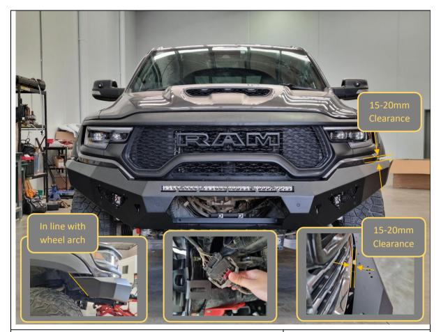
88. With assistance, from another person, align the bar with the edges of the vehicle. The bar should sit symmetric left/right on the vehicle.
