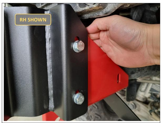
28. Loosely secure the inner face of each tow point to each impact assembly with 2x M10x25 hex bolts, flat washers and flange nuts.
