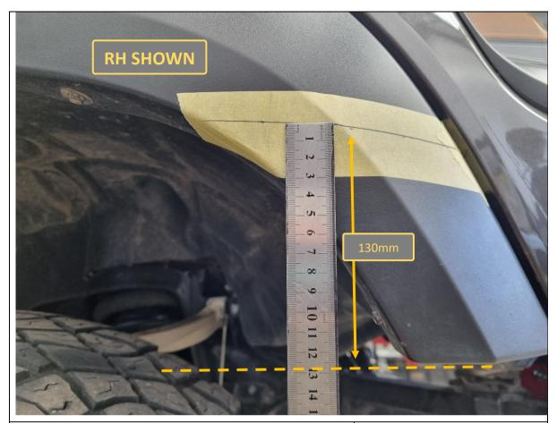
66. Measure and mark a straight horizontal line that is parallel to the bottom edge of the flare, 130mm away. Do this for both flares.
