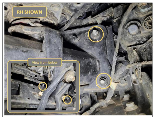
8. Remove 3x 18mm hex nuts (per side) holding the bumper to the chassis rail.
