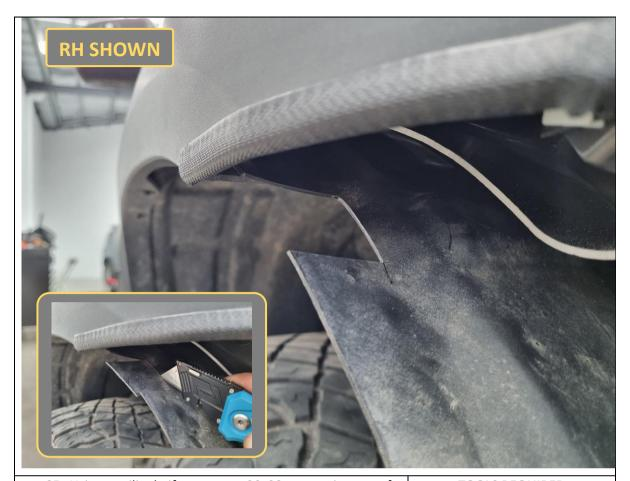
85. Using a utility knife, cut out a 30x30mm section out of the wheel arch liner, directly below the flare cut. Do this on both sides.
