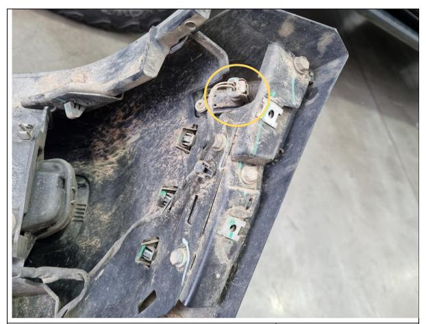
38. Unplug the side marker lamps located on the outer ends of the bumper. These lamps will not be relocated into the bullbar.
