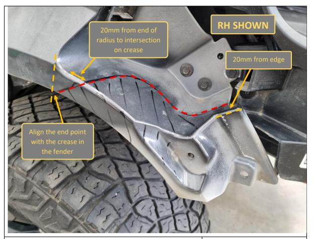
73. The fiberglass fender also needs a section cut and removed. Use a marker pen and ruler to mark out the cut area on the fender.
