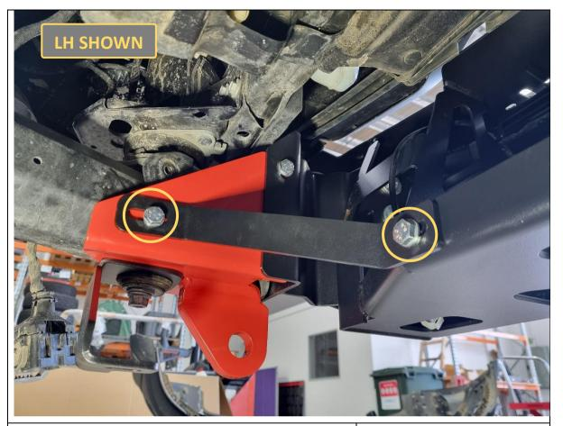
91. From underneath the vehicle, install the 2x tension straps connecting the bottom of the winch cradle to the tow points.
