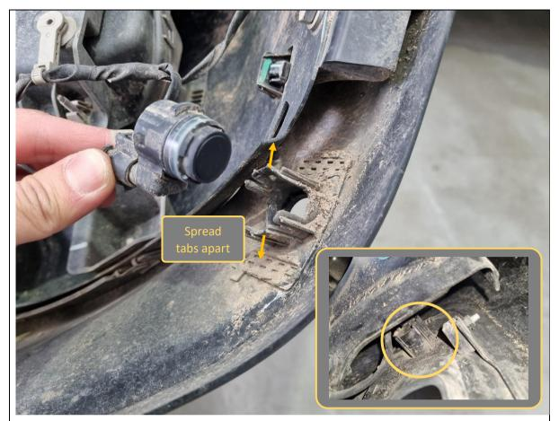
39. Locate the 6x parking sensors on the bumper, and unclip them from its plastic housing by spreading the housing plastic tabs apart.
