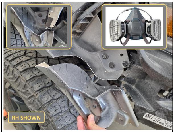
74. Use an air hacksaw to cut the fender along the marked cut line.
