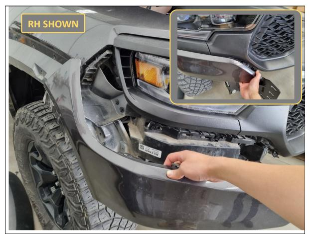
72. Remove the plastic trim under each headlight. Start at the base of the grille and pull the trim outwards to release the clips.
