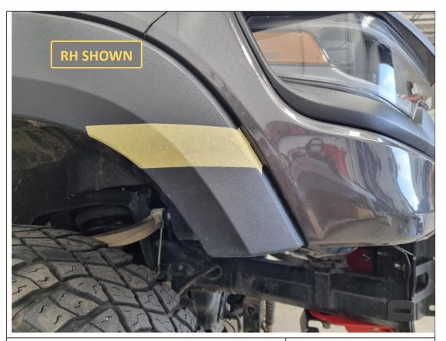
65. The wheel flares need to be trimmed to fit the bar. Apply masking tape over the flares in approximately the position shown.
