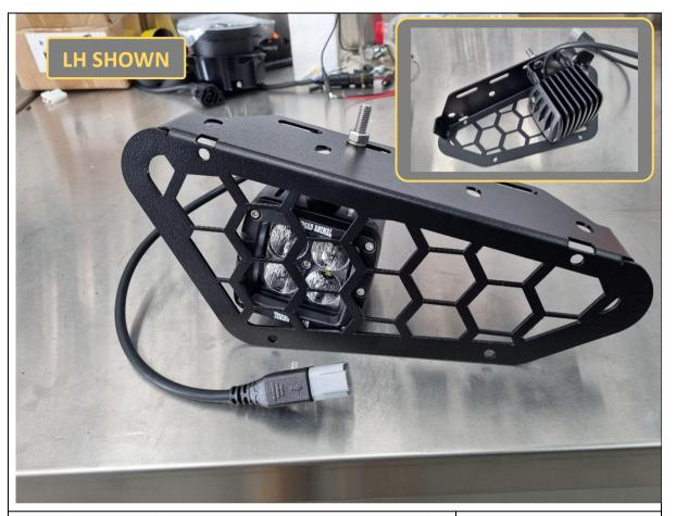
56. If wanting to fit other lights to the wing mesh instead of fog lights, do so now. The wing mesh is capable to taking most 8" light bars and cube lights.
