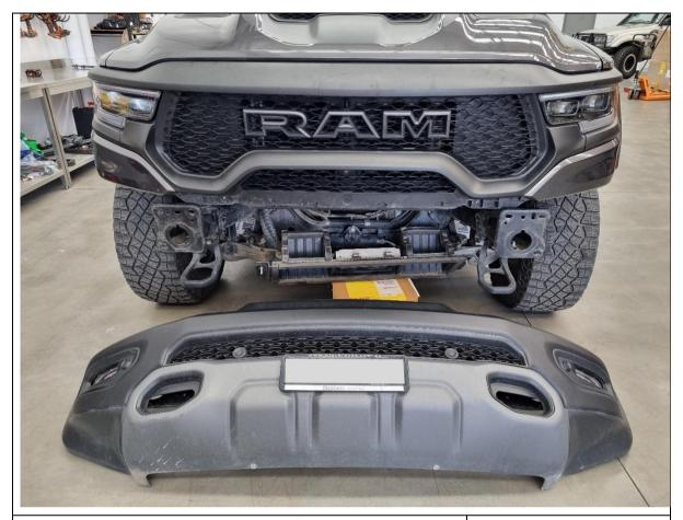
9. With a lifting device or assistance from another person, pull the bumper outwards and remove from the vehicle. Set the bumper aside in a safe place.
