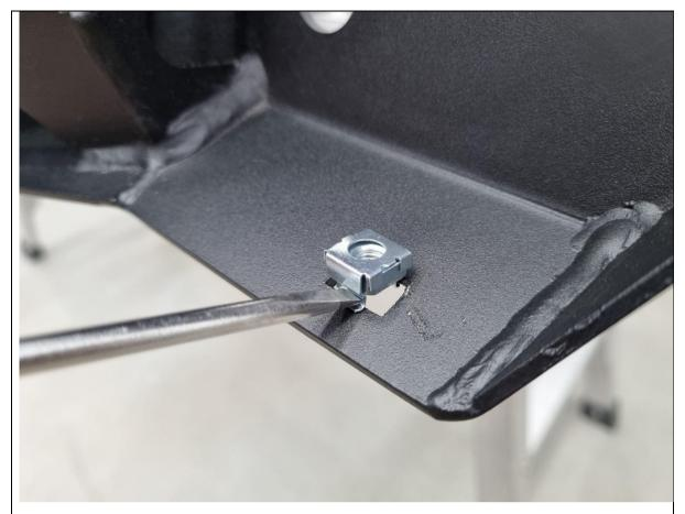
64. Fit 10x M6 cage nuts into the rectangular slots on the bottom of the bar wing (5x per side).
